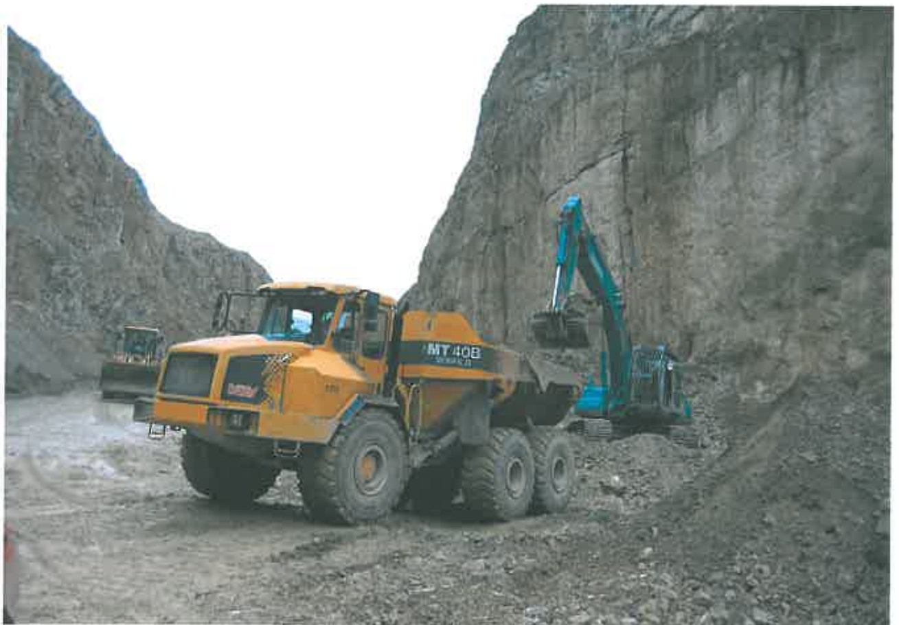
Figure 2 Working vein fluorspar in an open pit from the South Pennine Ore Field, Derbyshire, UK BGS@NERC.
